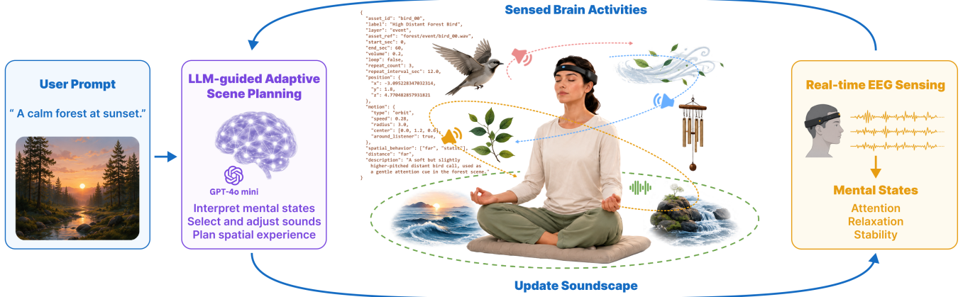
Figure 1: NeuroScape transforms spatial audio from a static meditation background into a responsive environment that adapts to users' internal states. The system combines user-guided scene initialization, EEG sensing, adaptive scene planning, and real-time spatial soundscape rendering in a continuous closed loop.
